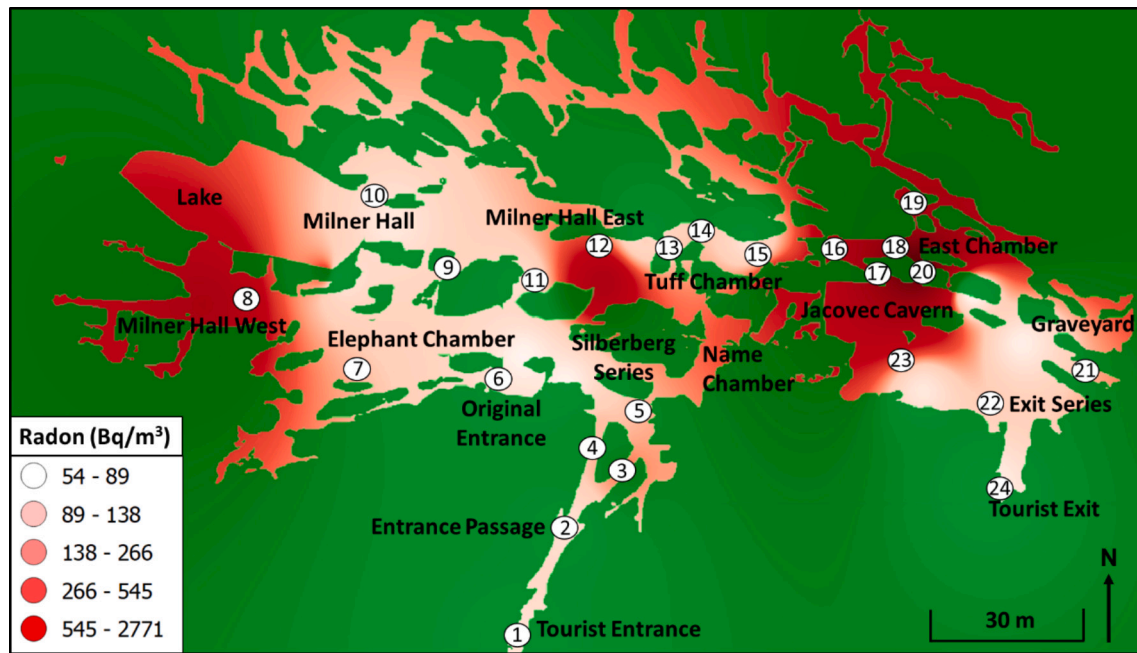
Fig. 2. A radon map of the Sterkfontein Cave with a graduated radon concentration overlay and the locations of the measurements indicated with numbers.
